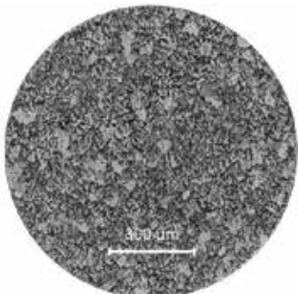
WAAM ER5356 @ MetalWorm Reference 5019 Aluminum alloy [5]
