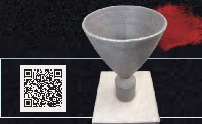
Rocket Nozzle ER316LSI Stainless Steel
