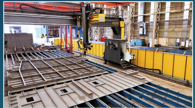
Web-Panel Manufacturing Line
